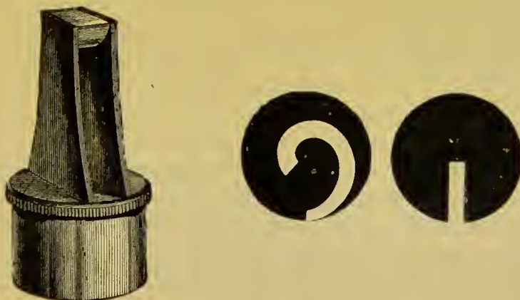
Fig. 142.—Mayall's Semi-Cylinder Illuminator and Spiral Diaphragms.
